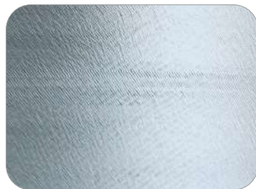
Surface with vibrations R_a = 0.7 \mu\text{m}
