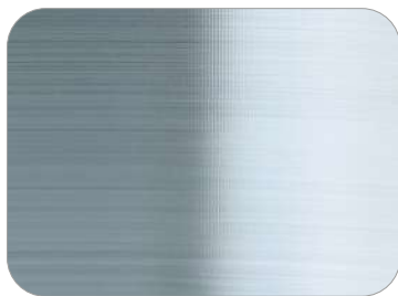
Surface without vibrations R_a = 0.35 \mu\text{m}
