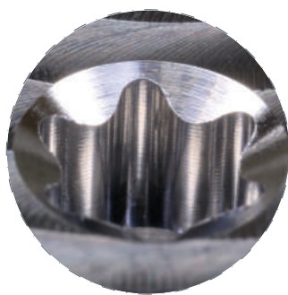
Machined Torx socket with REF 1450
