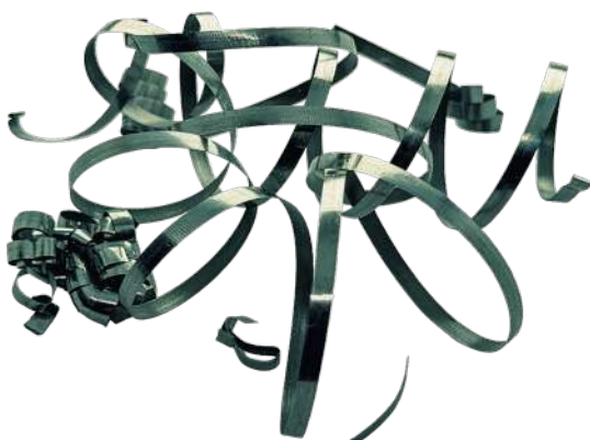
Einstechen ohne Spanformer (42CrMoS4+QT) / grooving without chipformer (42CrMoS4+QT)
